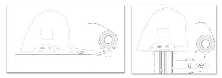
Release the Pinch Rollers by pressing down on the Pinch Roller Release Levers.
