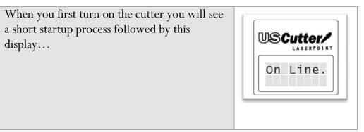
Press the  $\bigcup_{\text{Line}}^{\text{On}}$  Button to enter Off Line Mode to access the Off Line functions.
