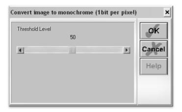
Now you can adjust the Threshold Level slider. Where you place the slider will determine how much of the image will be included in the monochrome conversion (*which is to become the image that will be cut*). Anything darker than the level set on the Threshold slider will be included in the cut and anything lighter will not.
