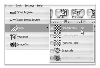
Sometimes an imported image will already be in monochrome but will still need to be vectorized before being cut. If the image imported is monochrome than you can skip ahead to the "vectorise" section.
