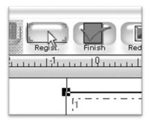
You will need to add registration marks on both the left and right sides of the bottom edge of the printed image.
