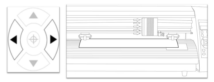
Now press the target key to tell the cutter that this is the location where you would like the cut to begin.
