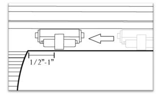
Engage the Pinch Rollers by pulling up on the Pinch Roller Release Levers.
