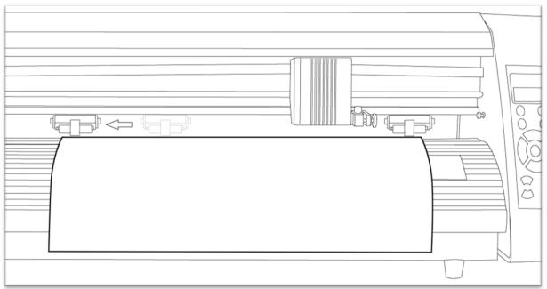
Leave a gap of between  $\frac{1}{2}$ -1 inch from the edge of the roller and the edge of the vinyl on both sides.
