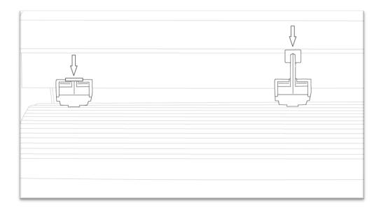
Feed the vinyl underneath the pinch rollers (*if working from a single sheet instead of a roll the vinyl can also be feed from the front*).
