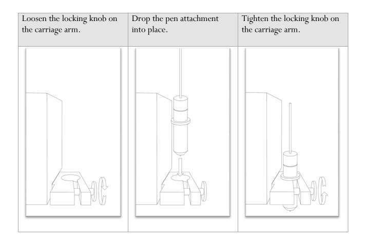
It may be easier to install the pen (or blade) carriage after the lid on the LaserPoint has been raised allowing more working room.
