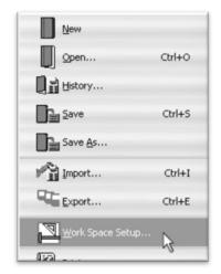
Now you can either select a preregistered work space size, or you can enter your own dimensions into the Height and Length fields. In this demo we are planning on cutting a single sheet of  $8\frac{1}{2}x11$  paper so we entered 11.00 into the height field and 8.50 into the length field.
