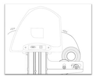
Adjust the pinch rollers from side to side so there is one roller on each side of the vinyl.
