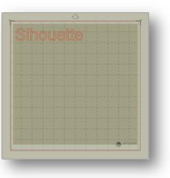
When viewing in this manner, the red line will still represent your cutting area. Images falling outside of this red cutting area will not be cut. The darker area on the cutting mat represents your printer's print margin area and is only for reference.
