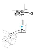
Lift up the needle-changing tool so that the fork hooks onto the needle clamp screw.
