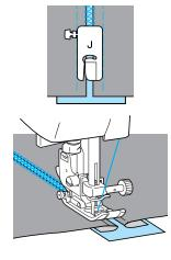
After sewing is finished, remove the paper.
