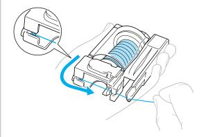
Pass the thread through the notch in the lower-right corner of the thread cassette, and then pull the thread to the left.
