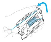
• When using special thread such as metallic thread, use the thumb of your left hand to lightly press down on the area indicated in the illustration to create an opening that allows for easier threading.
