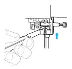
Insert the needle until it touches the needle stopper, and then use the screwdriver to tighten the needle clamp screw.
