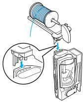
Thread the thread cassette with the thread from the spool on the extra spool pin.
