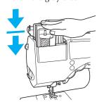
X Inserting the cassette partway and pausing before fully inserting it
