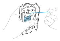
Pass the thread through the slit in the top of the thread cassette.
