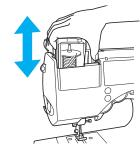
X Inserting the cassette only partway, then pulling it out
