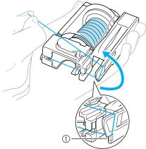
Pull the thread under the disc at the front in the lower-left corner and around to the right, and then the thread will be cut with the cutter. Follow arrow 6 indicated on the thread cassette.
