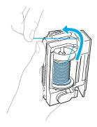
Pull the thread to the left and pass it through the slit along the left side of the thread cassette.
